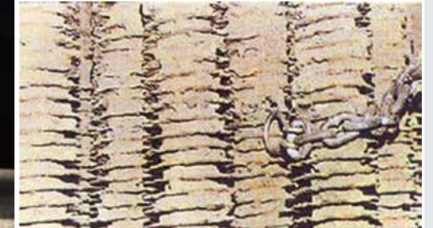
Helical finned tube after 4,000 hours operation
